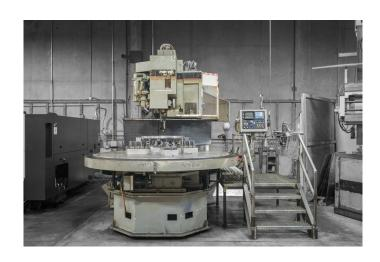
MONARCH 96" VMC-RT - CNC DRILLING MACHINE Drill holes 0.25" - 3" diameter Work piece: 20" - 108" diameter Ideal for: Drilling bolt holes
