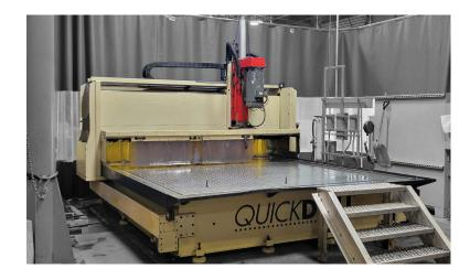
QUICKDRILL GANTRY MACHINING CENTER - CNC MILL 120" x 120" work envelope Ideal for: Drilling and milling large flanges- 8"in. thick and up to 18'ft. in diameter.
