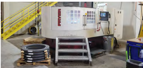
FRYER VT-80 - VERTICAL TURRET LATHE
