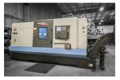
DOOSAN PUMA 480/GT3100-HORIZONTAL CNC LATHE Maximum turning diameter: .5" - 21.5" Maximum length of work: 39" Ideal for: High volume turning of complex parts
