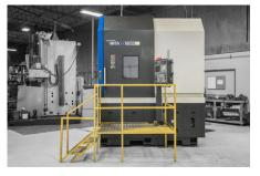
HYUNDAI WIA LV1100R - VERTICAL CNC LATHE Maximum turning diameter: 39" Ideal for: High volume turning of complex parts up to 39" diameters
