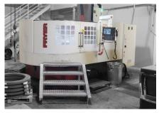
FRYER VT-80 - VERTICAL TURRET LATHE Max Cutting Length 32" Cutting Diameter Range 4"- 80" Ideal for: High volume turning of complex parts up to 80" diameter
