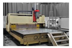
QUICKDRILL GANTRY MACHINING CENTER -CNC MILL 120" x 120" work envelope Ideal for: Drilling and milling large flanges- 8"in.
