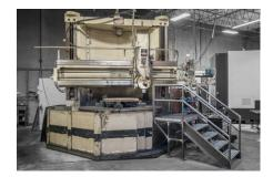
**BULLARD DYNATROL - VERTICAL TURRET LATHE** Maximum turning diameter: 108" I**deal for:** Turning rings and flanges with 42" to 108" outer diameter
