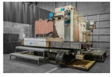
IKEGAI NB11T – HORIZONTAL CNC MILL Horizontal milling with 59" x 39" work envelope Ideal for: Multi-axis milling and boring
