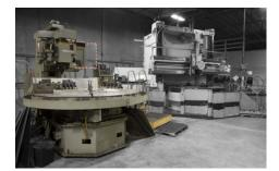
MONARCH 96" VMC-RT - CNC DRILLING MACHINE Drill holes: 0.25" - 3" diameter Work piece: 20" - 108" diameter Ideal for: Drilling bolt holes
