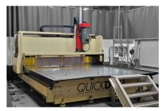
QUICKDRILL GANTRY MACHINING CENTER-CNC MILL
