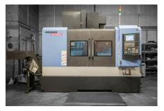
DOOSAN MYNX 5400/50 - CNC MILL 40" x 20" work envelope Ideal for: Precision drilling & milling
