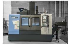
DOOSAN DNM 5700 - CNC MILL 40" x 20" work envelope Ideal for: High-speed milling of material such as aluminum and plastic
