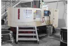
FRYER VT-80 - VERTICAL TURRET LATHE Max Cutting Length 32" Cutting Diameter Range 4"- 80" Ideal for: High volume turning of complex parts up to 80" diameter
