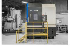
HYUNDAI WIA LV1100R - VERTICAL CNC LATHE Turning diameter: 22-39" Ideal for: High volume turning of complex parts up to 39" in diameter
