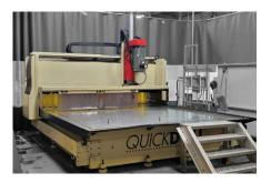
QUICKDRILL GANTRY MACHINING CENTER-CNC MILL
